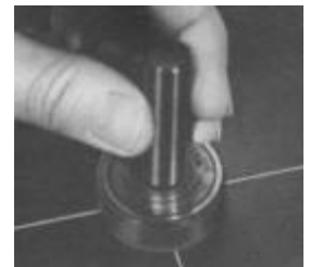
PRECISION CENTER PUNCH INSERTED IN CENTER-RITE BODY
