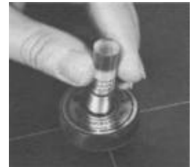
OPTICAL CENTERING GAUGE INSERTED IN CENTER-RITE BODY
